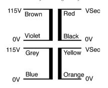
Primary 2x115V @ 50-60Hz Suitable for Series/Parallel connection
